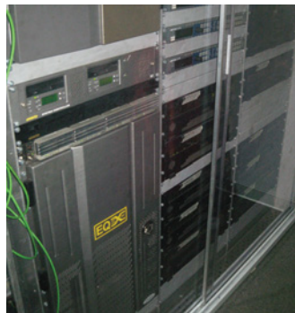
Already playing a key role on the truck, an Evertz EQX 288 high density SD/HD/3G router currently has a 128x128 configuration
