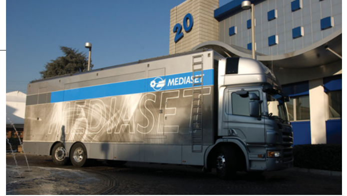
Raised edges, borders or external hinges have been reduced to a minimum so that more than 10 of overall 12m are dedicated to internal work space
